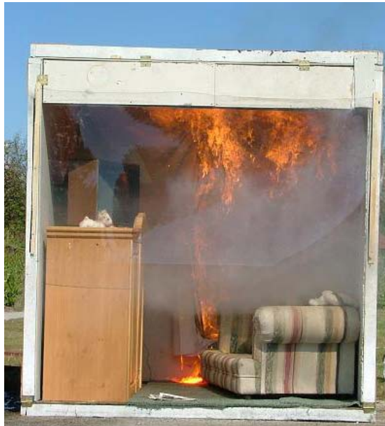
Non-sprinklered burn cell after approximately two minutes.
